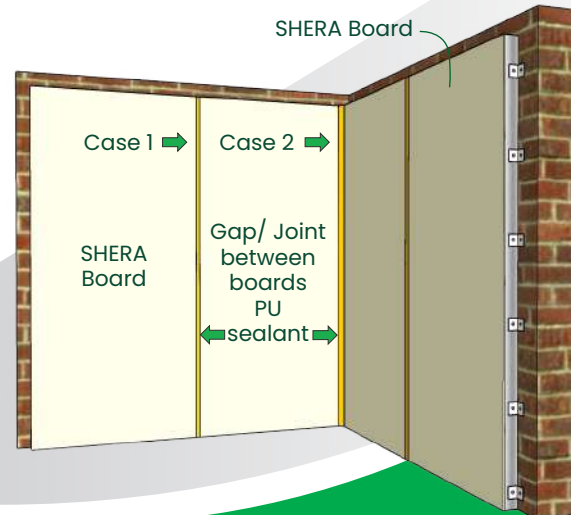
Case 2 L Corner Board to board joint
